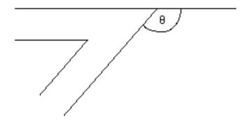
This gives 90° for bends A and C, 131° for bend B and 45° for bend D. Thus the order of difficulty of the bends is (from most to least difficult) B, A and C, D.
